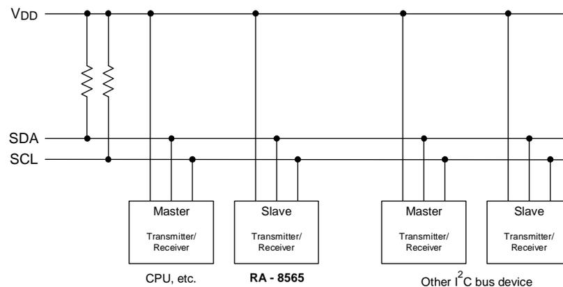
Any device that controls the data transmission and data reception is defined as a "Master". and any device that is controlled by a master device is defined as a "Slave".
