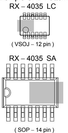
\* The shaded part ( ) indicates where a GND pattern should be set without getting too close to a signal line
