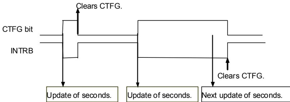
Note: When Clock Precision Adjustment Function works, a period of interrupt changes by that quantity of the adjustment once per 20 seconds or one minute.
