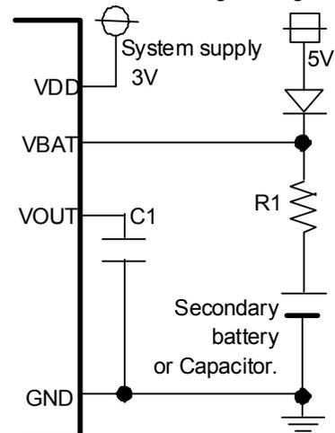
8.4 Note of battery switch-over circuit.
