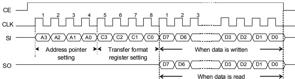
\* There are two transfer methods each for read and write operations.
