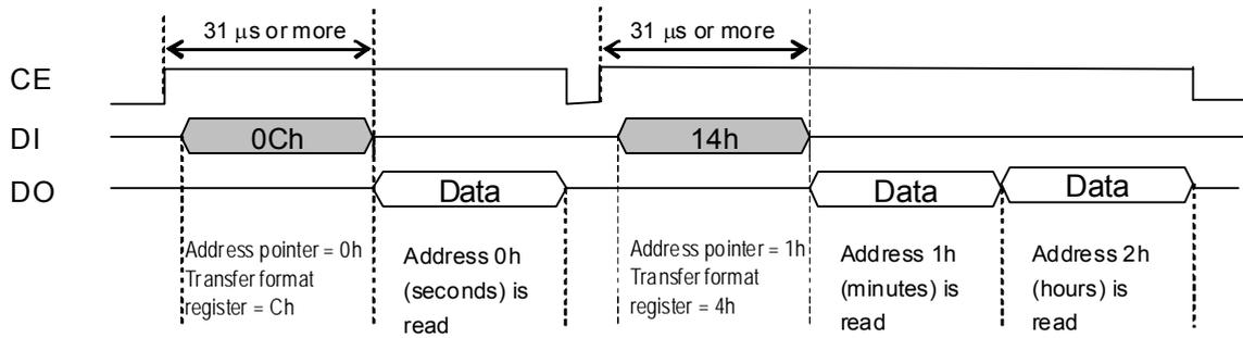
Incorrect example 2: If interval is less than 31  $\mu$ s when time write operation is started
