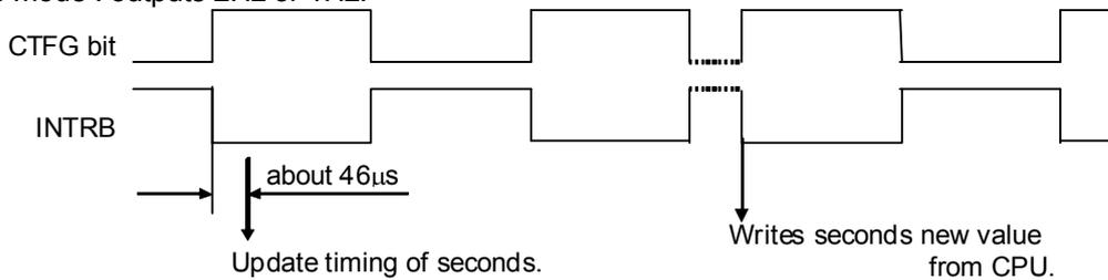
In a pulse mode, update of seconds is behind with about 46µs from a falling edge of INT.
