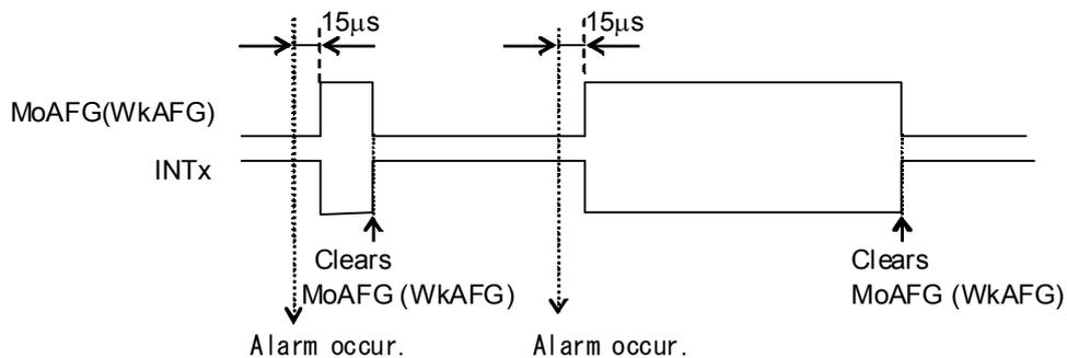
9.6.2 Alarm\_Wk register (BANK=0 Address 8-Ah)
