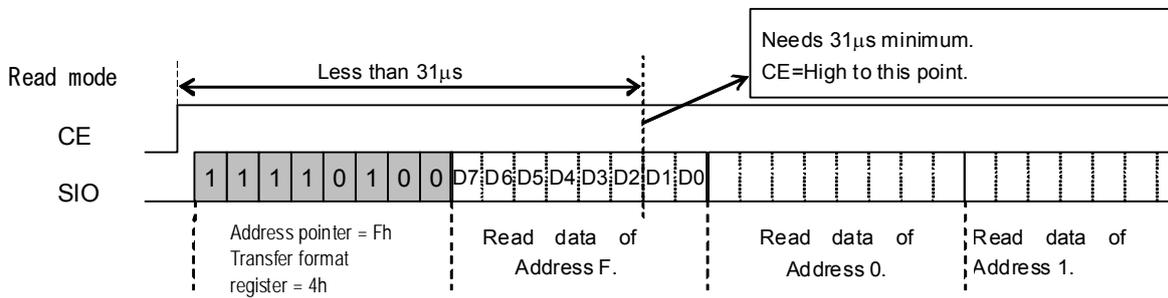
Incorrect example 3: If interval between two time read operations is less than 61  $\mu$ s
